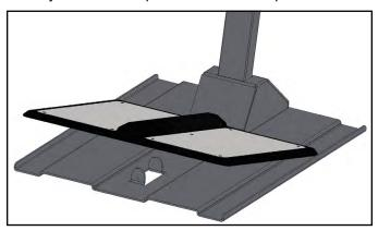
Figure 7. Installing the dual foot plate onto the baseplate
