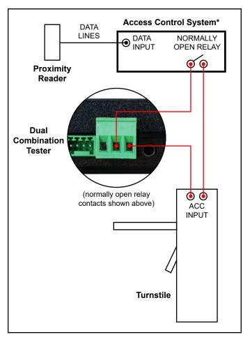
Figure 8. Wiring the Dual Combination Tester to an Access Control System
